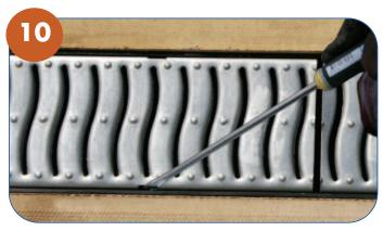
✓ Insert a screwdriver into the slots provided, twist and lift to remove the grate.
